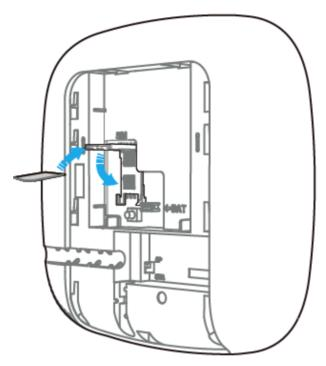
Figure 3-2 Insert SIM Card
