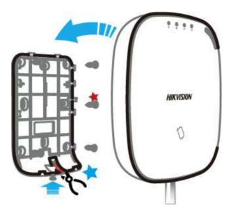
Figure 3-6 Complete the Installation
