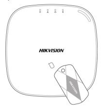
While the system is not armed, present a valid card to the control panel to arm the system. While the system is armed, present a valid card to the control panel to disarm the system. The card operations and responding voice prompts are shown below.
