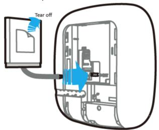
Figure 3-3 Connect the Battery
